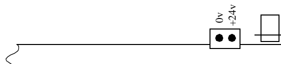
Figure 13. Power Connector Placement
